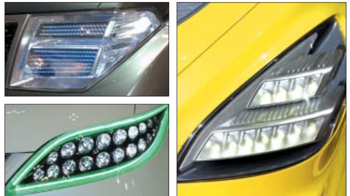
Fig. 4. The lower output power of LEDs dictates a multi-element headlamp design. Credit: Fausto Bigi and Jean-Paul Charret, Valeo Signals and Lighting.
