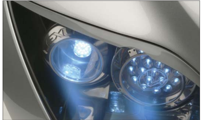
Fig. 2. The Lexus LF-C concept car features an all-LED headlamp (right) that has a highlighted Lexus logo on the inner lens.
