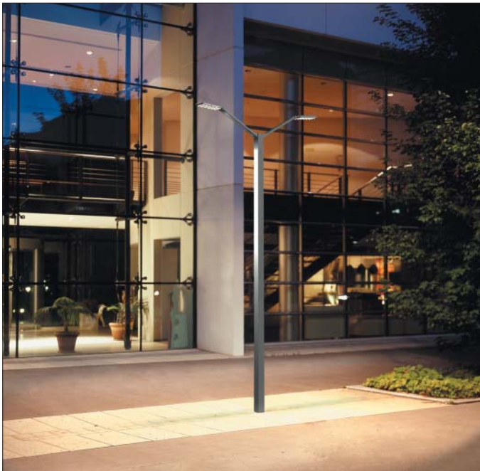
Fig. 5. The Equinox luminaire, designed to illuminate pathways, squares and shopping areas, contains 18 white and amber Luxeon I and III LEDs in each optical unit, combined with 'meniscus' optics.
