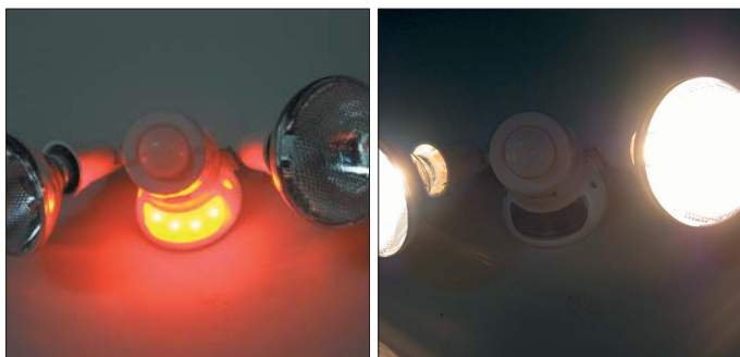
Fig. 3. This hybrid security light developed by Watt Stopper contains a 5 W amber LED array providing continuous illumination (left), while an occupancy sensor turns on the incandescent flood lamps when motion is detected (right).
