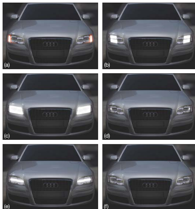
Fig.1. Could the Audi Allroad concept become the first production car to feature all-LED headlamps? The lights are fully roadworthy and have been put through countless tests and road trials. The different functions are as follows: turn-signal (a), low-beam headlights (b), high-beam headlights (c), parking lights (d), daytime running lights (e), and lights off (f).
