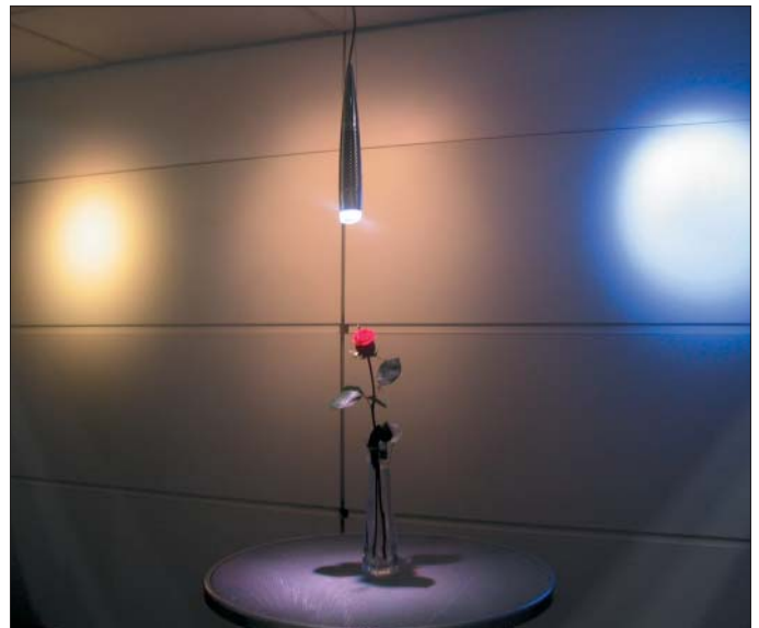
The spot in the center background is from a 50 W quartz halogen PAR 30 fixture, while the side spots are from 35 W LEXEL luminaires. The left spot is from an RGB LEXEL light set to about 2800 K (LEXEL provides CCTs in the 2000–6000 K range), and the right spot is from a dimmable white LEXEL. In the foreground, an RGB LEXEL LED module illuminates a rose, which did not wilt over a four-day period.
