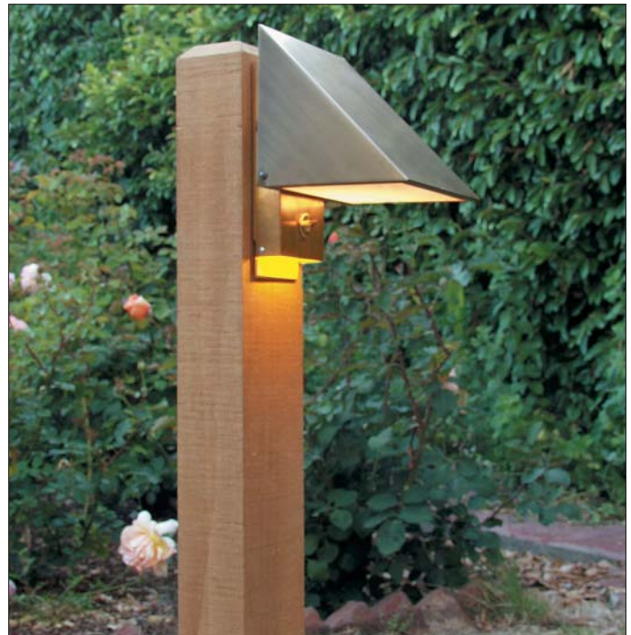
Fig. 1. In this hybrid LED/incandescent outdoor fixture developed by California Lighting Technology Center and partners, a 5 W LED array burns continuously and a 75 W incandescent lamp turns on at a signal from an occupancy sensor.
