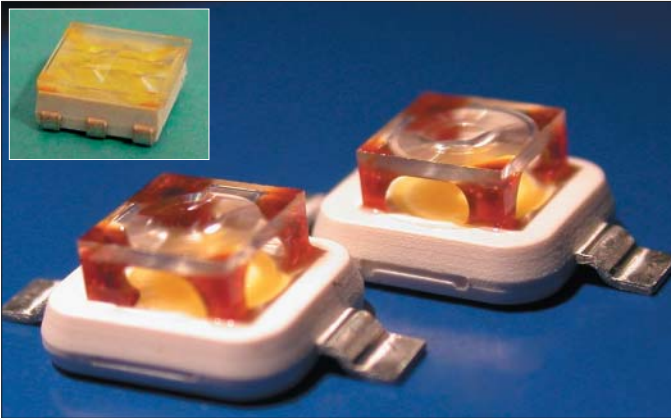
Fig. 4. Beam-shaping elements with a replicated DOE, assembled using replicated mounting pins. Inset shows latest version.
