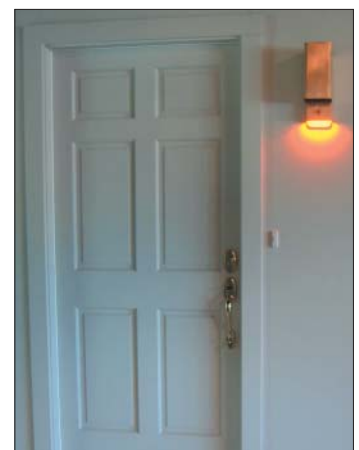
Fig. 2. The amber LED used in this hybrid porch light fixture is a good match for the popular yellow "bug lights" used on many porches.
