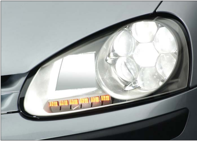
Fig. 2. Hella's earlier LED-headlamp prototype, demonstrated on a VW Golf, achieves a luminous flux of nearly 1000 lm in the low beam. The headlamp recently won a top award for innovation at the Barcelona Motor Show.
