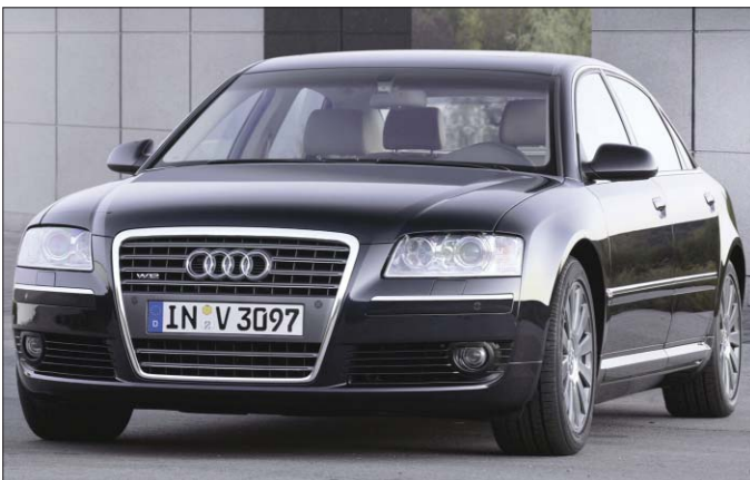
Fig. 4. The Audi A8 W12 has a daytime running light comprising five white Luxeon LEDs in a distinctive clover-leaf pattern.
