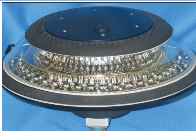
Fig. 4. Fuselage-mounted anti-collision lights utilizing high-power LEDs. (Courtesy Jeff Singer, Honeywell.)
