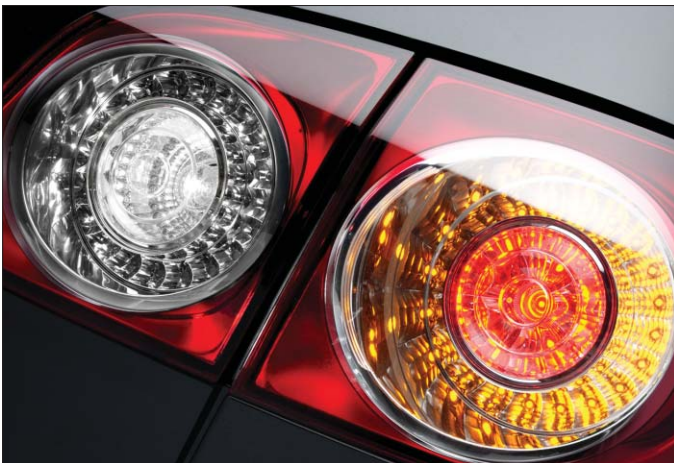
Fig. 3. Hella has supplied rear combination lamps (RCLs) for the VW Golf Plus. Each outer lamp has two concentric rings containing a total of 36 red and red-amber LEDs. Different combinations of these LEDs create the tail lights, brake lights and indicators.
