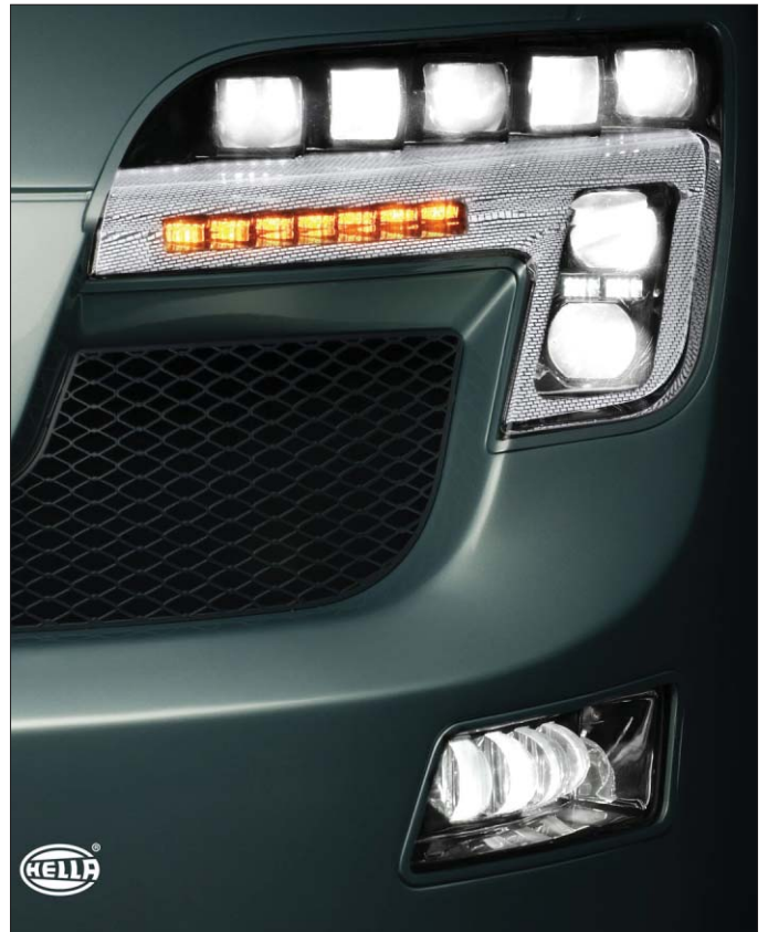
Fig. 1. The prototype LED headlamp developed by Hella and Stanley features seven Cartoval lenses in front of multi-chip white LED arrays which provide the low- and high-beam functions. A homogeneously illuminated white "LED curtain" acts as the position light, while a dynamic bending light is incorporated into the bumper.
