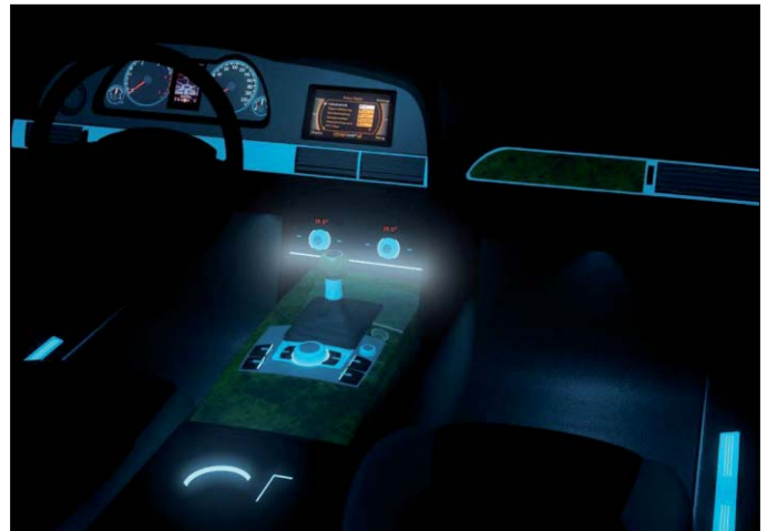
Fig. 1. The car interior of the future? Ambient lighting in vehicles can enhance the driver's comfort and orientation while providing brand identity for the vehicle manufacturer. (Courtesy of Delphi.)
