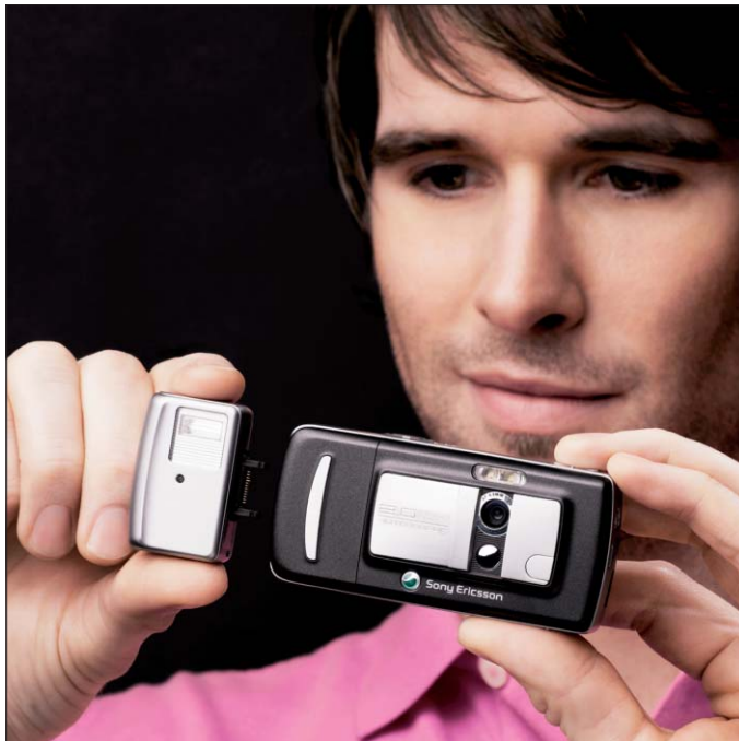
Fig. 4. Sony Ericsson's K750i handset has a 2Mpixel camera and two high-power LEDs to provide additional illumination for low-light conditions. However, the company also sells an add-on xenon flash unit for "proper" photography.
