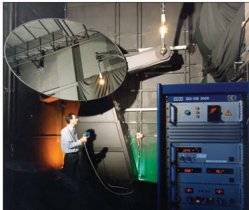
Fig. 1. NPL's reference goniophotometer.
