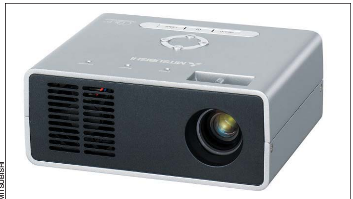
Fig. 2. Mitsubishi's second generation LED-based PK-20 PocketProjector™, launched in June 2006, has an ultra-wide lens enabling users to create a 20-inch diagonal screen with just over a foot of projection distance. The suggested retail price is $899, with the battery pack costing a further $199.
