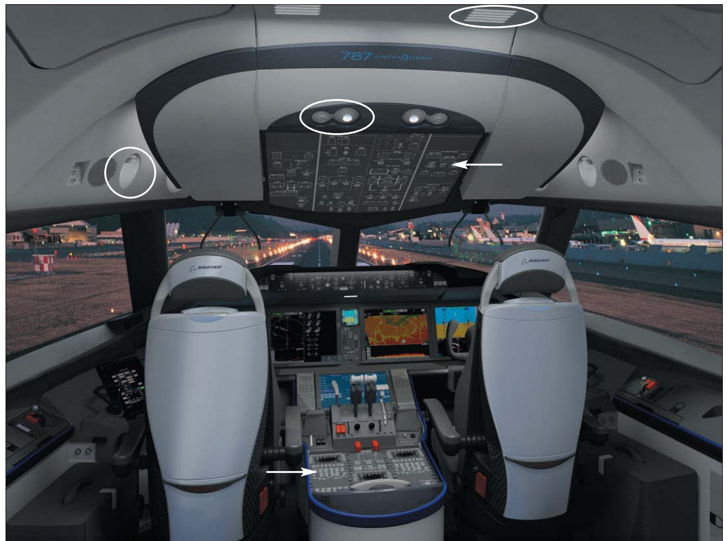
Fig. 1. Boeing 787 cockpit, showing some of the white LED lighting systems supplied by Goodrich (circled) and back-illuminated panels supplied to Korry by IDD Aerospace (arrowed).
