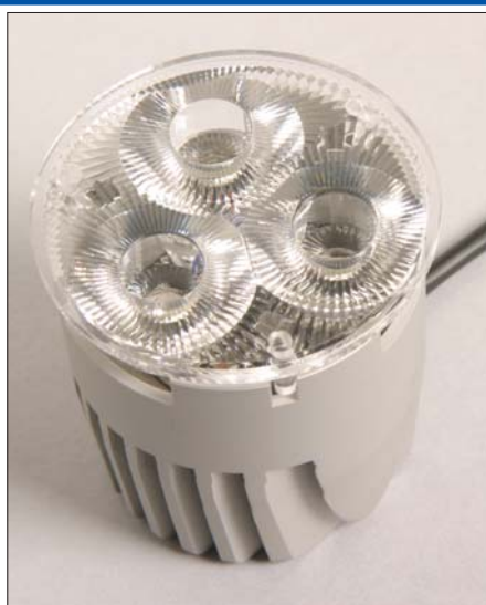
Fig. 2. Dialight-Lumidrive has built modules with on-board drivers for low-voltage applications that eliminate electrolytic capacitors and incorporate thermal feedback.
