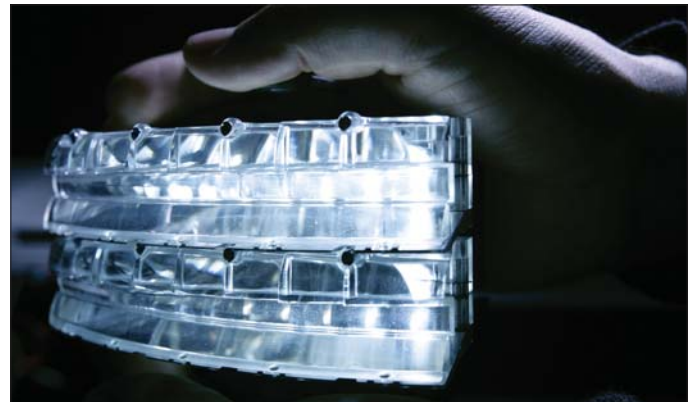
Fig. 3. Audi Le Mans concept car with LED headlamps designed by Ruetz, a German engineering company, using Optis software (see www.sae.org/automag/techbriefs/07-2004/1-112-7-52.pdf ).
