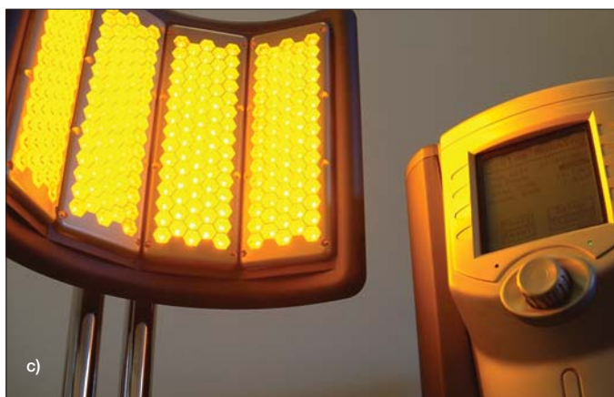
Fig. 1. LED-based systems from Enfis Ltd designed for various dermatological treatments: (a) a portable LED treatment device for use in the home; (b) a very high power-density system for use in a hospital or doctor's surgery; (c) a wide-area illumination system intended for use by doctors or in spas and health centers.
