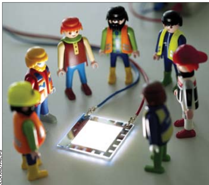
High-quality white light is emitted by OLED materials without phosphor conversion, as shown in this Philips demonstrator.
