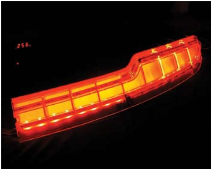
Tail-light assembly showing the illuminated spacers that form the amber turn signal.
