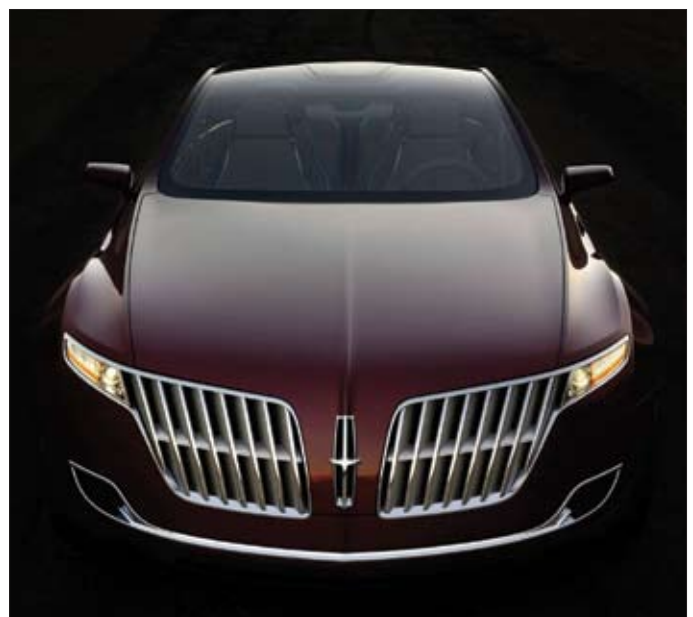
LED front lighting on the MKR includes a unique amber turn signal constructed with a lightguide bent around the headlamp.
