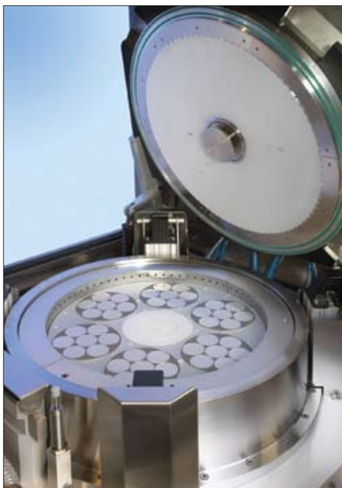
The new G4 machine from Aixtron can grow LED structures on 42 two-inch wafers in every run.
