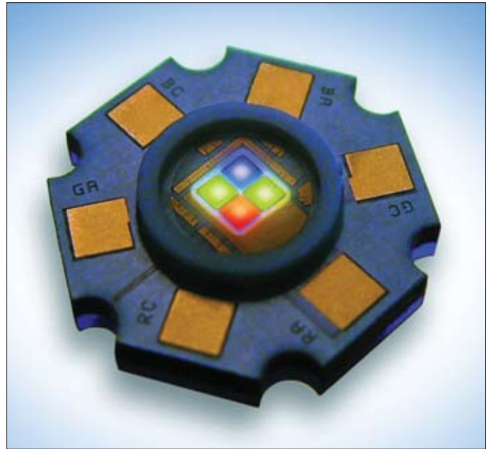
Fig. 1. PerkinElmer’s ACULED (all color ultrabright LED) high-performance RGB LED in COB technology.
