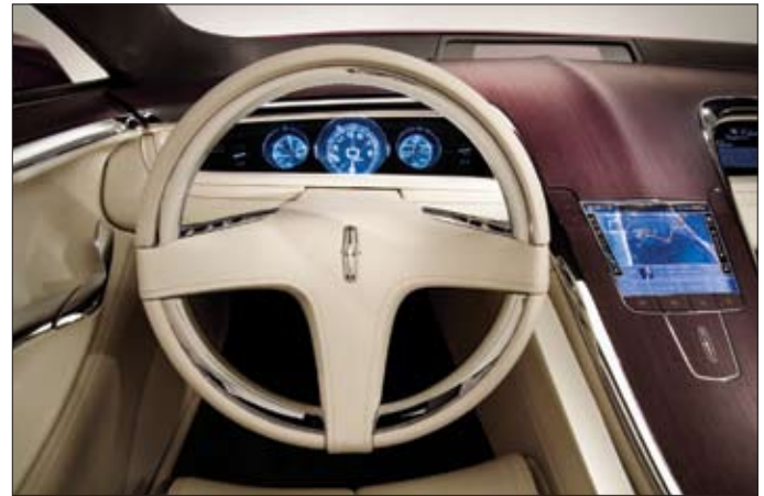
Acrylic lenses, LBW and LEDs create a dimensional look to the instrument cluster in the MKR concept.
