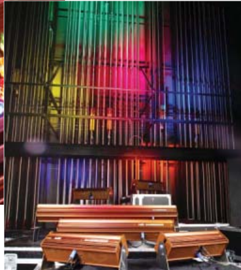
Figs. 3 & 4. The Selador X7 LED fixture uses a seven-color system to achieve a wide spectrum of colors that include the pastel range.
