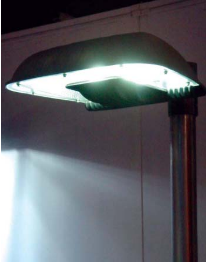
Fig. 10. Advanced LEDs: Hall 5.0 featured a good selection of LED outdoor lighting luminaires, including the Barracuda from Advanced LEDs Ltd. The LEDs (in this example, 5 arrays of 16 Cree XLamps) are mounted on the nose section and directed upwards, so that the light hits the reflector and produces the required distribution pattern. Heat pipes carry heat to the fins at the rear, while the whole nose section containing LEDs and drivers can be removed for maintenance if necessary. Photo courtesy of Carl Gardner.
