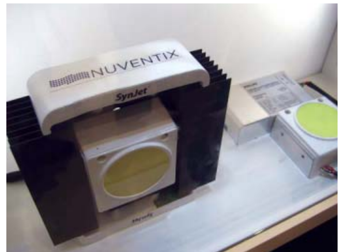
Fig. 6. Philips Fortimo module cooled by SynJet technology.
