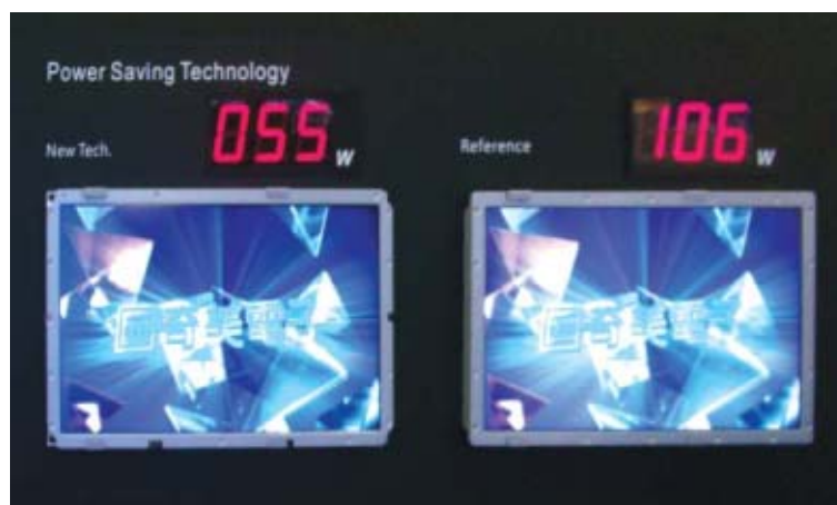
FIG. 5. Chi Mei Optoelectronics demonstrated LED backlight advantages over CCFL using side-by-side comparisons.
