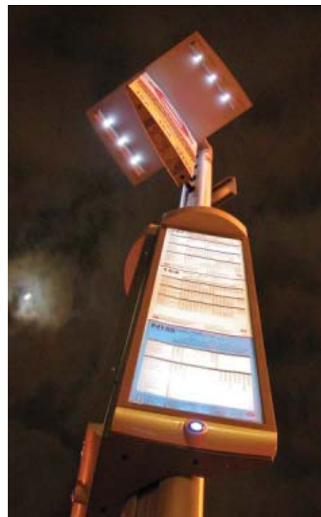
FIG. 4. Solar-powered transit stop provides LED down lighting, edge-lit schedule illumination, and user-activated signal light.
