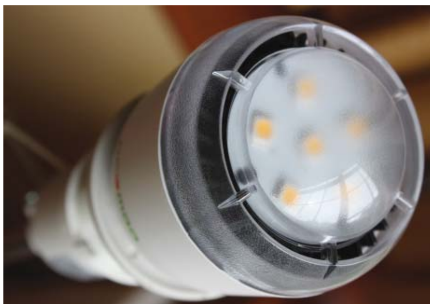
The EL1001 warm-white lamp from Ecomaa Lighting (Jhubei City, Taiwan) is rated at 510 lm and consumes 10 W. The company states this is equivalent to a 60 W incandescent, with an 80% energy saving. The lamp contains 6 LEDs from Nichia.
