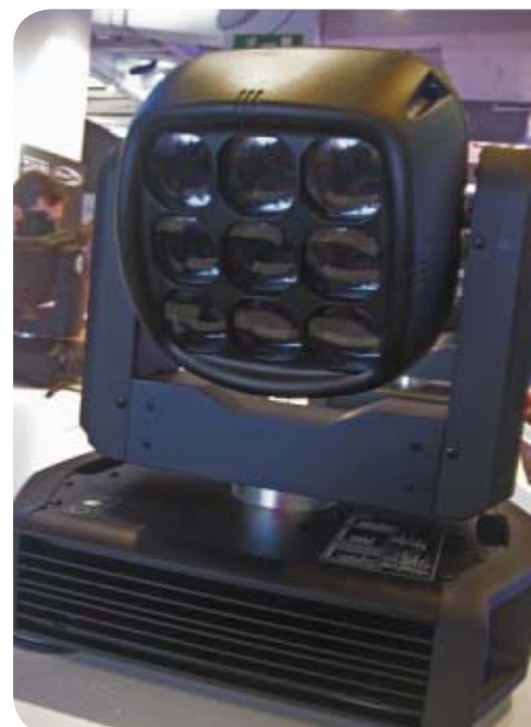
▲ The Tracker 300 from Showtec contains 9 LEDs that can be driven at 1400 mA (6W). Each LED can operate independently. The beam angle is 5 degrees, and the luminaire can produce 18,200 lux at a distance of 1 m.
