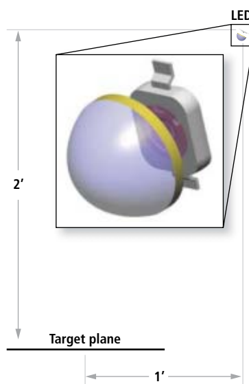
FIGURE 1. A simple task light can often be accurately modeled without taking the near-field light distribution into account.
