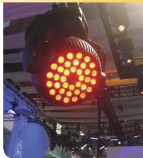
▲ The MAC 401 Dual from Martin is a LED-based moving head washlight with a beam-reflective mirror on the rear.
