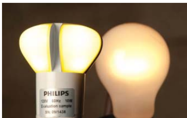
FIG. 3. The Philips DOE L-Prize candidate utilizes aluminum air channels for cooling and includes four separate LED modules that radiate light in most directions.
