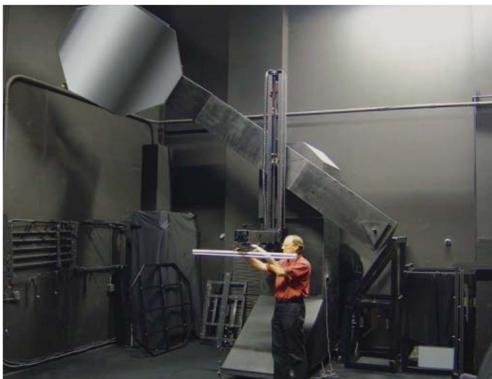
FIG. 1. LSI goniophotometer in the testing laboratory.
