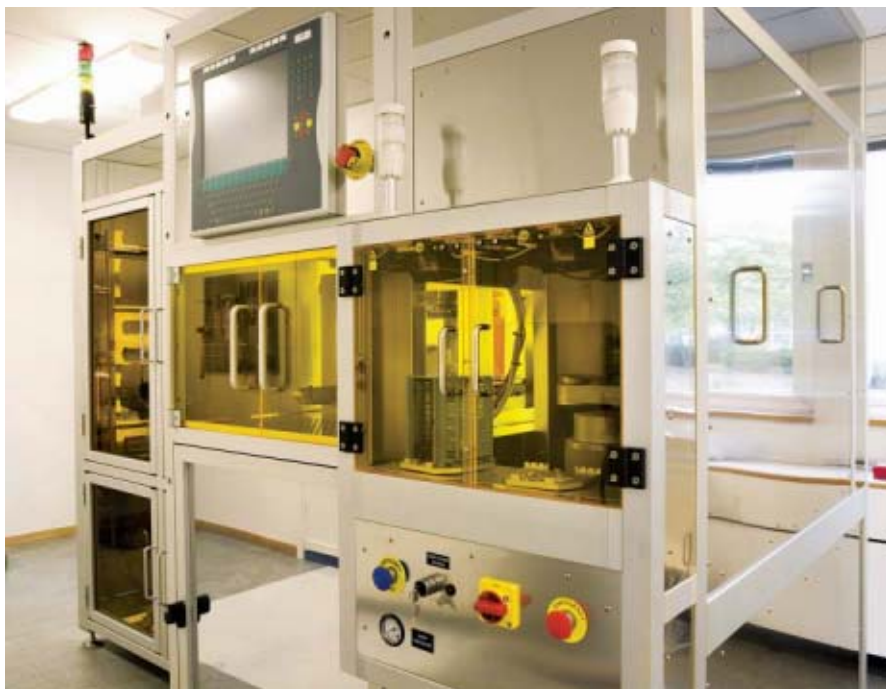
FIG. 2. High-volume Sindre nanoimprint lithography (NIL) manufacturing tool.
