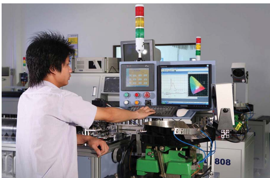
FIG. 1. Miniature spectrometers perform well in LED sorting operations, where rapid data acquisition and measurement accuracy are critical.
