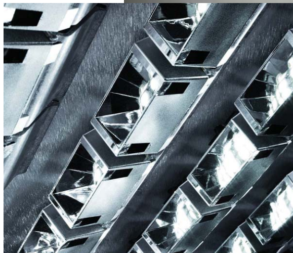
FIG. 5. The Kim street light mounts small groups of LEDs inside a MicroEmitter reflector module (inset) that directs light to a larger reflector to form the desired beam pattern.
