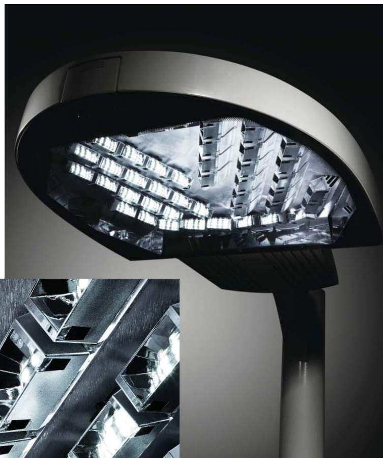
FIG. 5. The Kim street light mounts small groups of LEDs inside a MicroEmitter reflector module (inset) that directs light to a larger reflector to form the desired beam pattern.
