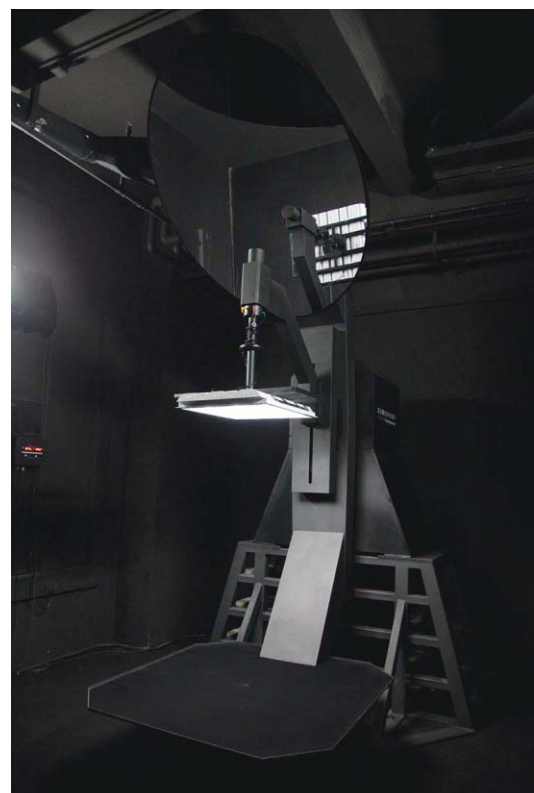
FIG. 1. A Type-C goniophotometer at UL's Nansha, China facility.
