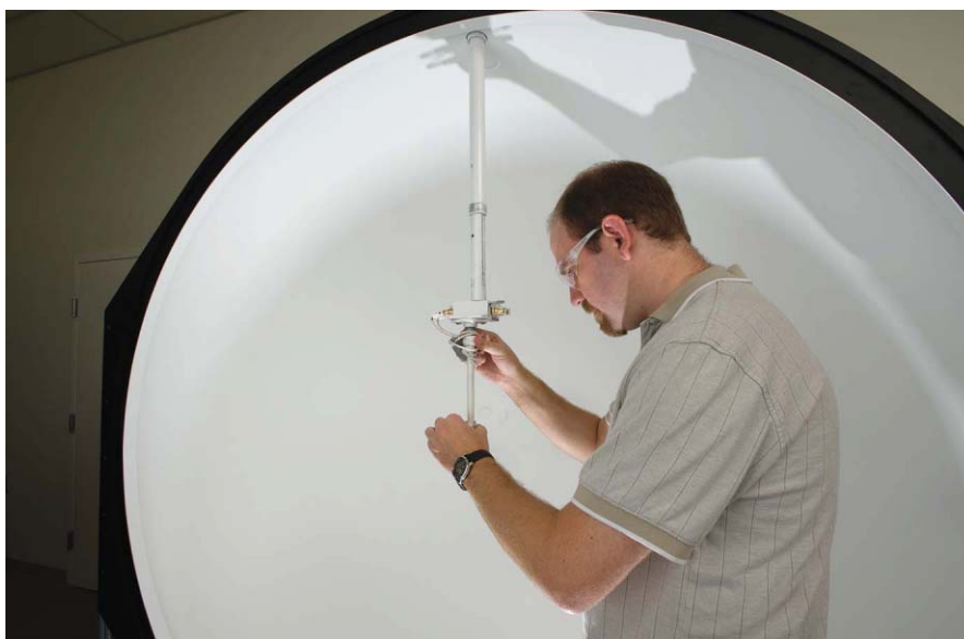
FIG. 2. An integrating sphere at UL's Luminaire Testing Laboratory facility.
