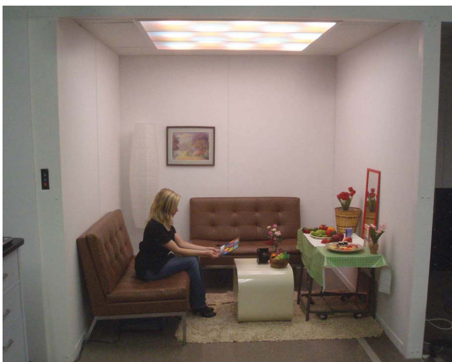
FIG. 1. NIST has a spectrally-tunable lighting lab with 22 color channels that enables research into color rendering.
