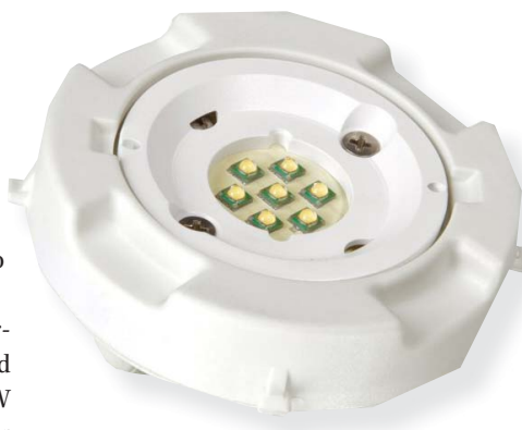
FIG. 4. GE Lighting has introduced new versions of its Infusion module, which can be connected to a socket in the luminaire body with a simple twist-lock mechanism. Three color temperatures – 2700K, 3000K and 4000K – are available, each with 4 different light outputs. At 3000K, different modules offer 1100 lm (15W, using 7 LEDs), 1500 lm, 2000 lm or 3000 lm (46W, using 22 LEDs).
