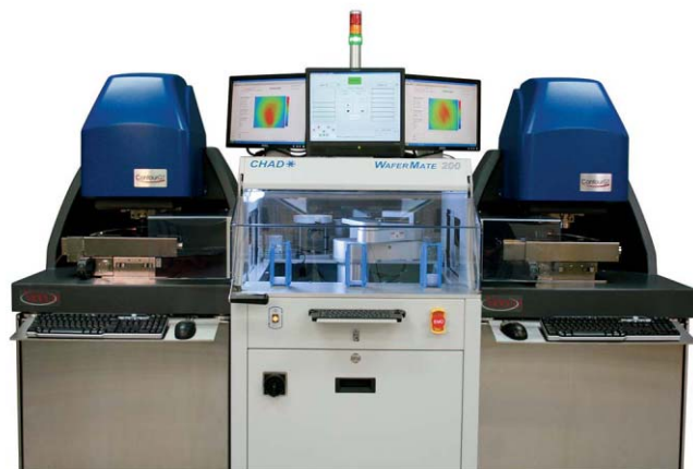
FIG. 5. A dual white-light interferometer (WLI) implementation with integrated wafer handling for the sapphire substrates speeds production testing.
