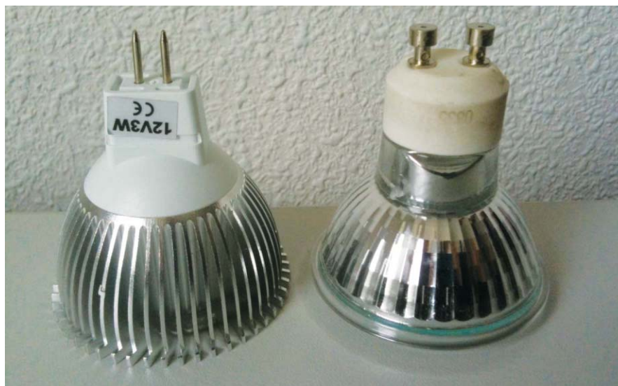
FIG. 1. A low-voltage, 3W, LED MR16 with GU-5.3 pins (left), and a 230-VAC, 50W, halogen MR16 with GU-10 pins (right).
