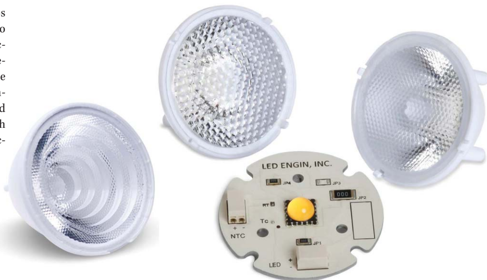
FIG. 1. TIR lenses and compact, high-lumen-density emitters from LED Engin. The company manufactures four compact emitter packages: 1-die up to 5W, 4-die up to 15W, 12-die up to 40W, and 24-die up to 80W.
