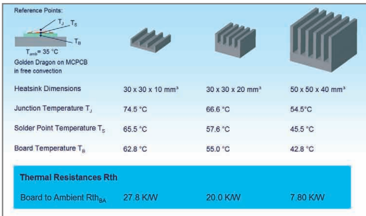
Figure 15: Thermal Resistance R_{thBA} of different heat sinks
