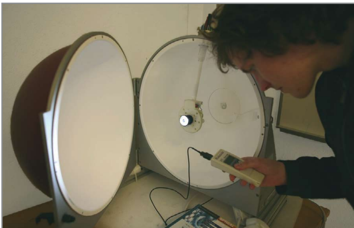
Figure 1: Measuring efficiency of a lens takes place in an integrating sphere.
