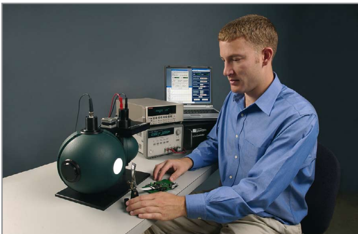
Figure 1: Traditional light measurement with integrating spheres.
