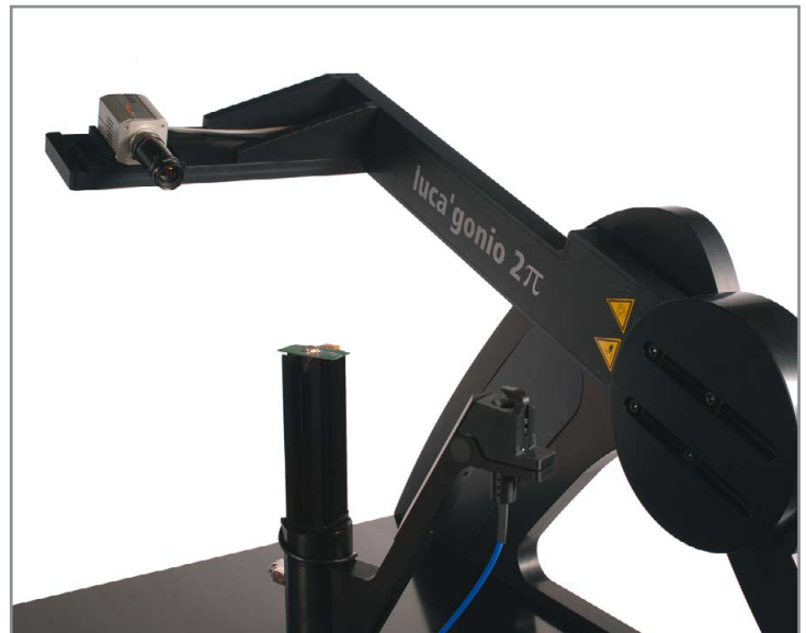
Figure 1: Near field source imaging goniometer.
