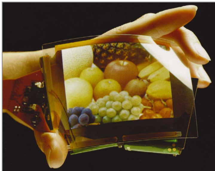
Figure 2: OLEDs are recognised as the best candidates for flexible displays.
