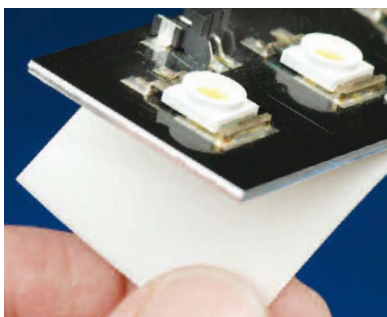
Thermally conductive insulated metal substrate boards specifically configured for LED applications.
