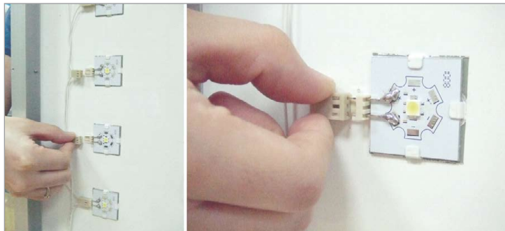
HPI's patented LED module systems allow easy replacement.
