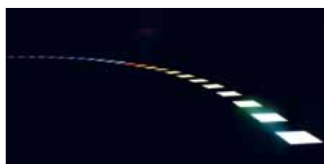
Verbatim’s color changing OLEDs showing the color tuning capabilities
