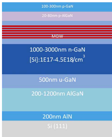
Figure 1: Different layers of the GaN-based LED stack
