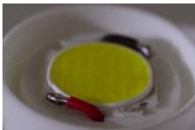
Figure 4: TA-I's ceramic substrate for replacement bulbs with E27 socket
