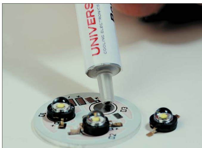
Packaged LEDs bonded to a metal PCB using thermal adhesive.
