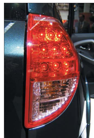
Fig. 2. The rear lamp on the new Toyota RAV4 SUV features nine LEDs for the brake function.
