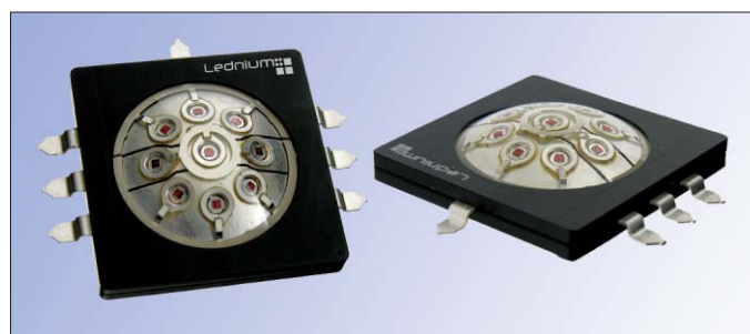
Fig. 1. With a unique dome-shaped package, the 10 W Lednium LED produces 250 lm in white at a current of 1.05 A. Excluding leads, the package size is 33 × 33 mm, and the height is 8 mm.
