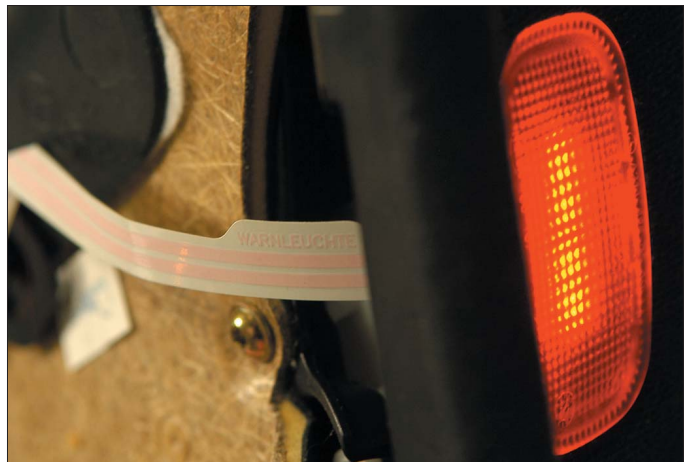
Fig. 5. Delphi’s low-profile lighting employs Flat Wire connectors.
