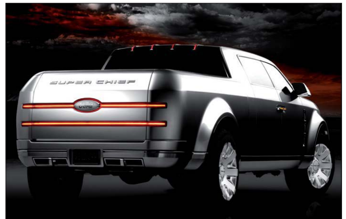
Figure 1. The front of the Ford Super Chief concept has white LED forward and fog lights, as well as amber “transparent chrome” running lights on the roof. The front indicator and door handle lights are made with LED light guides. The rear features horizontal light guides, as well as multiple LED brake light units on the roof.
