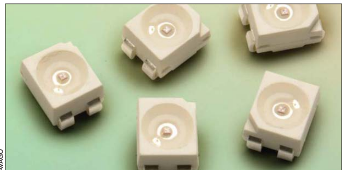
Fig. 4. Avago introduced the industry’s smallest 0.5 W LEDs at electronica. The new Envisium LEDs produce 6.6 lm and 9.3 lm in red-orange and amber, respectively, with a current of 150 mA. The package, a direct replacement for industry standard PLCC-4 packages, has two dummy leads to assist with heat extraction and measures 3.2 x 2.8 x 1.9 mm. The junction-pin thermal resistance is 60 °C/W, compared with 100 °C/W for the PLCC-4 package.
