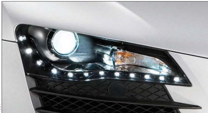
Fig. 1. Audi is vying with Lexus to bring the first car with LED headlights ( www.ledsmagazine.com/articles/news/3/10/23 ). The headlights for the Audi R8, featuring a distinctive curved line of LEDs for the DRL, were supplied by Germany's Automotive Lighting. The company says that this new LED headlamp incorporates more than 20 innovations in areas such as thermal management and control electronics, and that it has received special permission from the European Commission for the series application of LED headlamps in road traffic.
