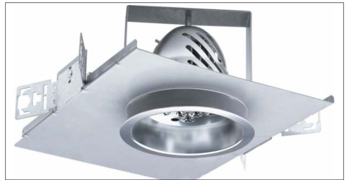
The Architektur D6LED downlight is built round a light engine comprising 10 white Luxeon K2 LEDs, each with a parabolic reflector, providing very uniform light output.
