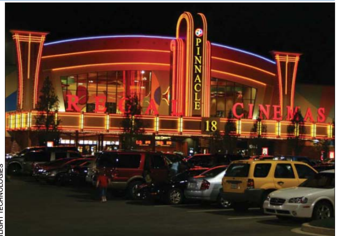
Fig. 7. LED linear lighting can replace neon in signage applications. The Regal Cinema in Knoxville, TN, uses more than a mile of LED exterior trim and accent lighting, supplied by iLight Technologies.
