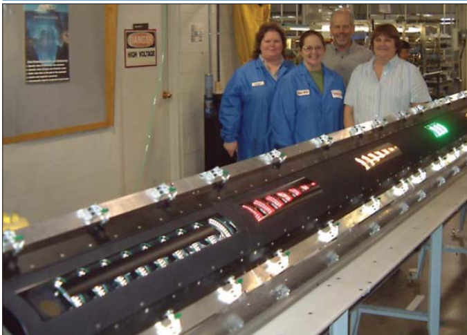
Fig. 6. This light, one of two sections of a pilot director light, is fixed to the underside of a refueling tanker aircraft to guide the incoming receiving pilot. The sections are 22 ft long and contain 3000 LEDs.
