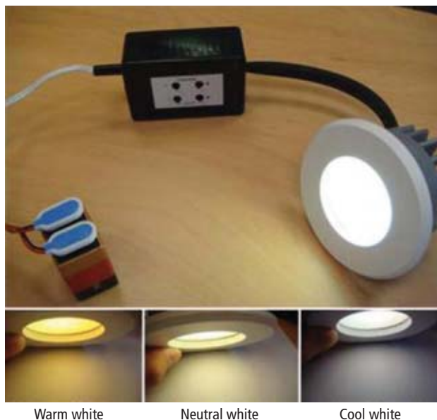
FIG. 2. Color-changing capabilities of the ChromaWhite LED module embedded in a standard PhotonStar CeilingStar5 recessed downlighter with a CCT and intensity controller box. The luminaire is running off two 9V batteries.
