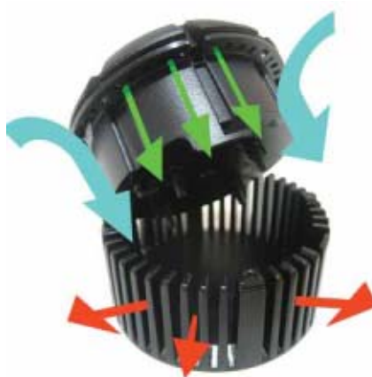
FIG. 4. Nuventix has supplied SynJet cooling modules to a number of luminaire manufacturers. A black SynJet and heat sink (left) are attached to a Fortimo light engine from Philips. Synthetic jets (right) are created by rapid-fire pulses of turbulent air produced by an oscillating diaphragm.
