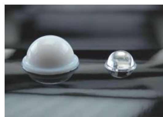
FIG. 3. Gel body (left) and final glass lens (right) with small mounting flange to fix the lens in a housing.
