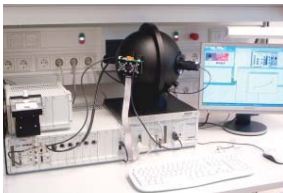
FIG. 2. Automated LED testing station combining thermal and optical test systems.
