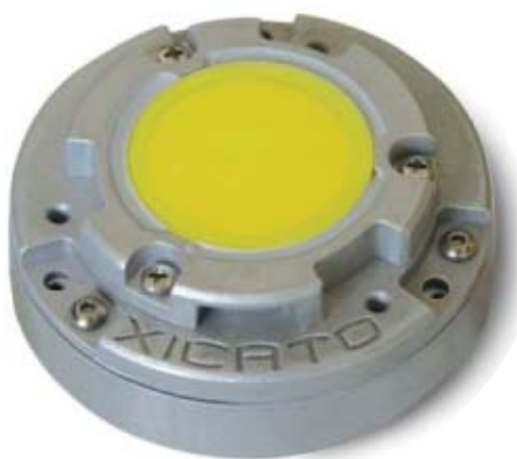
FIG. 1. The Xicato Spot Module (XSM) has a fixed form-factor with 48 mm diameter. Fixed outputs are 400, 700 or 1000 lm at 700 mA, at 9, 15 and 22W respectively. The outputs are similar to 20, 35 and 50W halogen lamps respectively. As LED efficacies improve, fewer LEDs will be needed and the module efficacy will improve, but the form factor and optical interface will stay the same. All technical data is taken at a recommended operating test point (Tc) temperature of 70°C.
