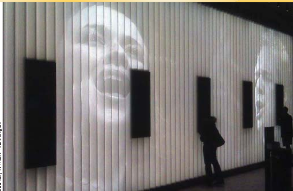
FIGURE 2. The David H. Koch Theater at Lincoln Center in Manhattan features an LED installation using the Traxon 1PXL Board Warm White, which illuminates cut Corian material from behind. The dual-view cut Corian with Traxon's Boards creates static grayscale images of a ballet dancer from one angle and opera singers from another angle.
