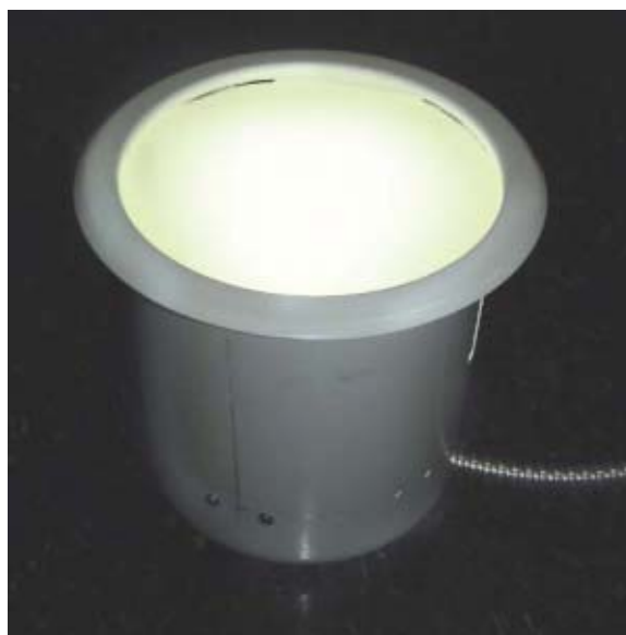
FIG.1. This LED downlight prototype has redundant optical design – the only impact of the failure of one single LED is a reduction in total light output.
