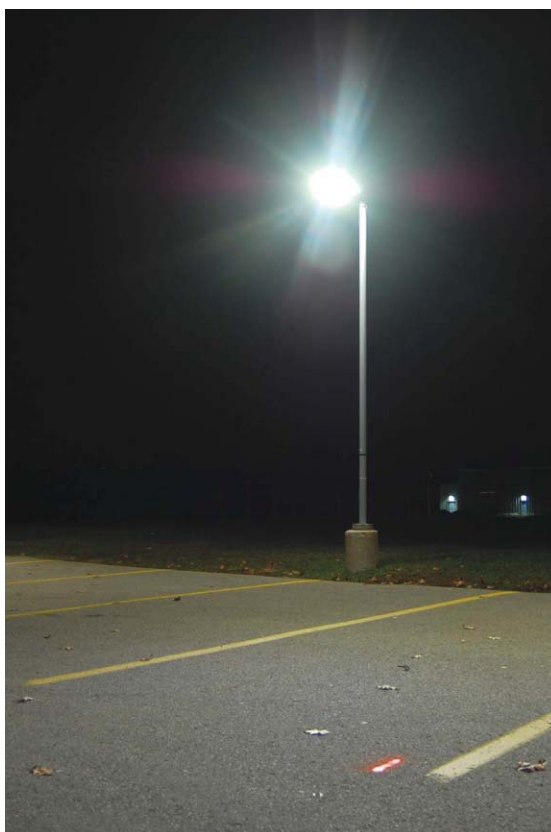
FIG. 1. One of the Elumen LED street lights with a illuminance measurement location marked in red on the pavement.
